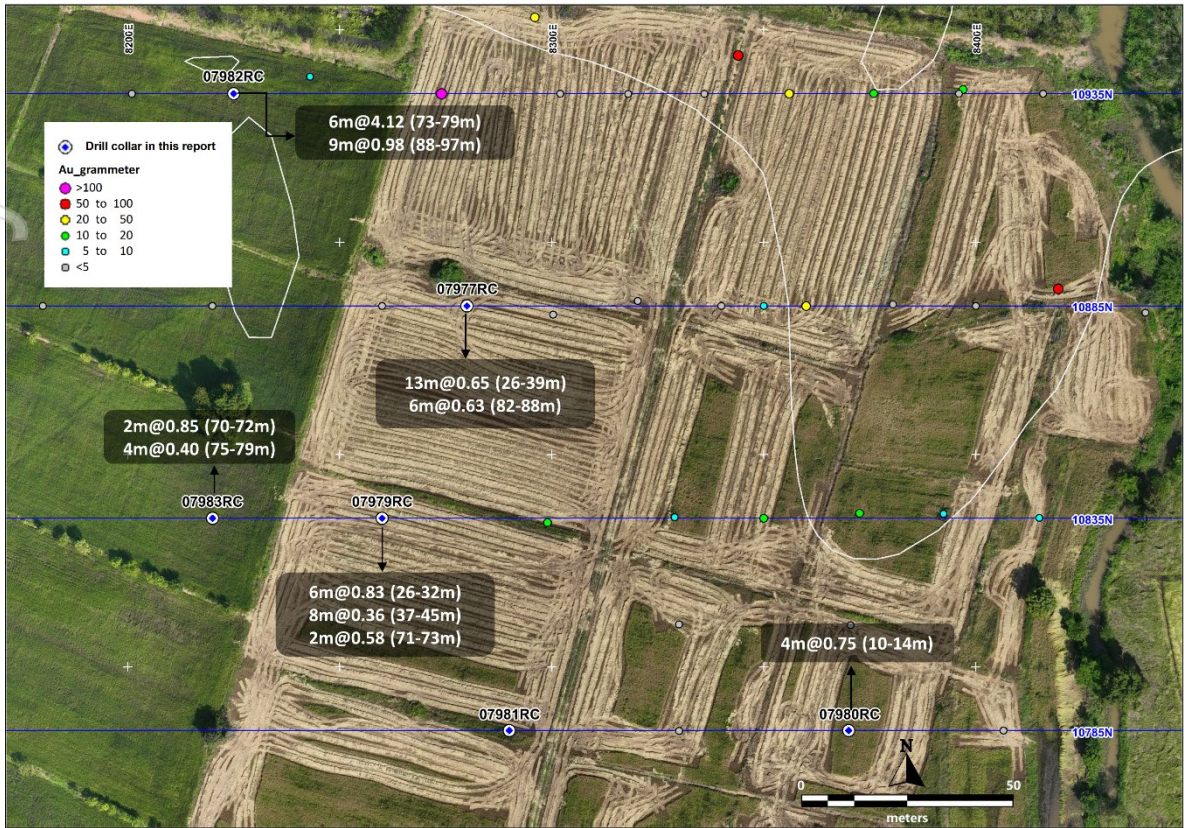
Figure 3: Drill hole locations and gold assay highlights 9 testing the western limb and southern continuity of the northern expression of the anticlinal structure 10
