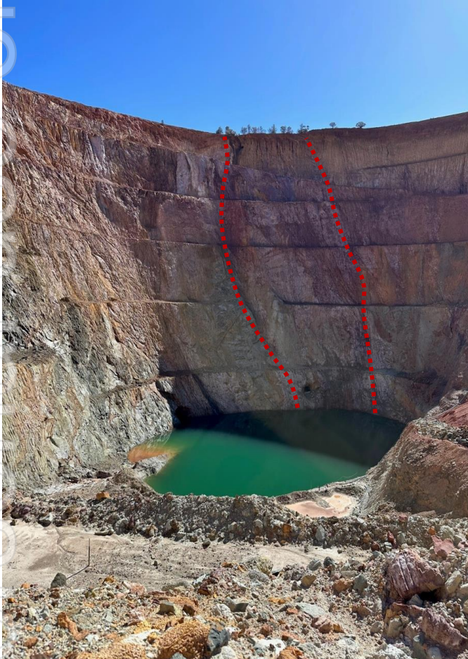
Figure 2 – Eureka Open Pit North Wall showing gold ore zone within shear zone
