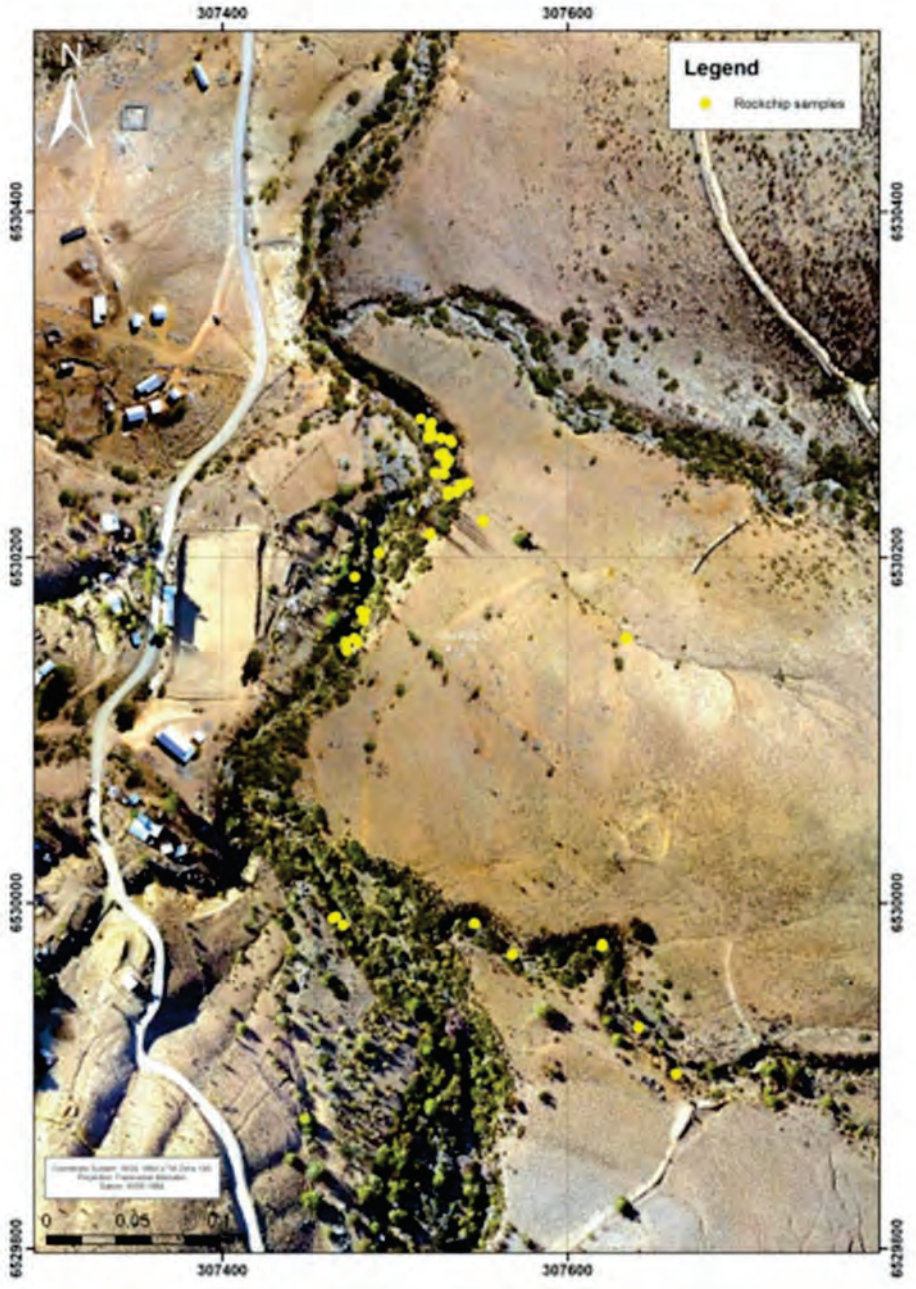
Figure 10. Rock samples from new target East Porphyry east of the Ferro deposit, mostly covered by colluvium so largely blind to geochemistry.
