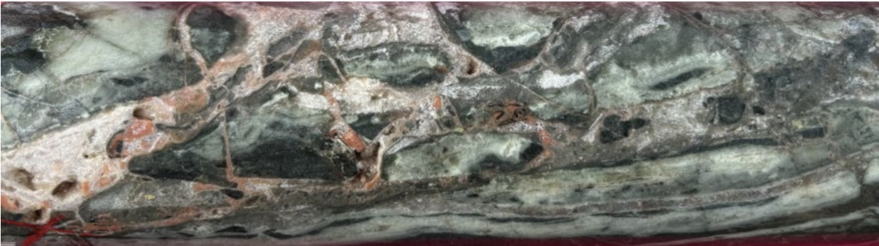
Figure 9: PP-GRAV01 diamond core drill holes intersected intensely hydrothermally altered, veined and brecciated Malu Formation meta-sediment, host to both Telfer and Winu, and some felsic intrusives. Prevalent alteration types were albite, K-spar, silica, quartz, calcite and haematite. Prevalent veining and breccia matrix types were quartz, calcite, haematite and Fe-oxides. Drill core photographs top to bottom 24PTDD003 from 148.3m, 24PTDD003 from 145.0m and 24PTDD003 from 182.5m. NB: Scale = NQ diamond core diameter 48mm.
