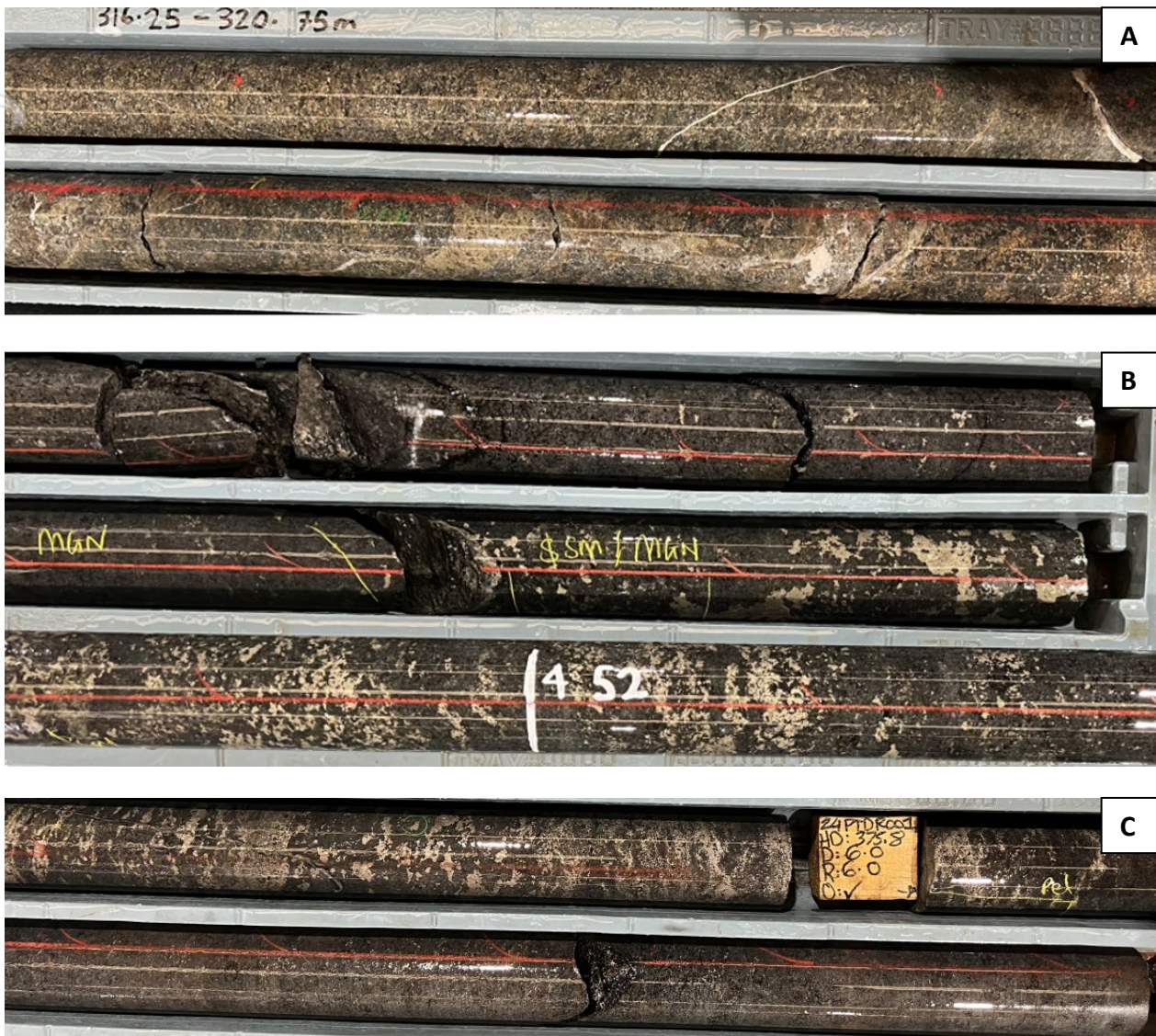
Figure 7A-C: PP-GRAV02 diamond core drill hole 24PTDR001 potassic altered (biotite-amphibole-chlorite \pm minor K-spar, albite and calcite) mafic intrusive (dolerite) hosting variable zones of disseminated, semi-massive, brecciated pyrrhotite-pyrite-chalcopyrite copper mineralisation. 24PTDR001 drill core photographs A from 316 to 318m, B from 450.5 to 452.5m and C from 375.5 to 377.5m. NB: Scale = NQ diamond core diameter 48mm.
