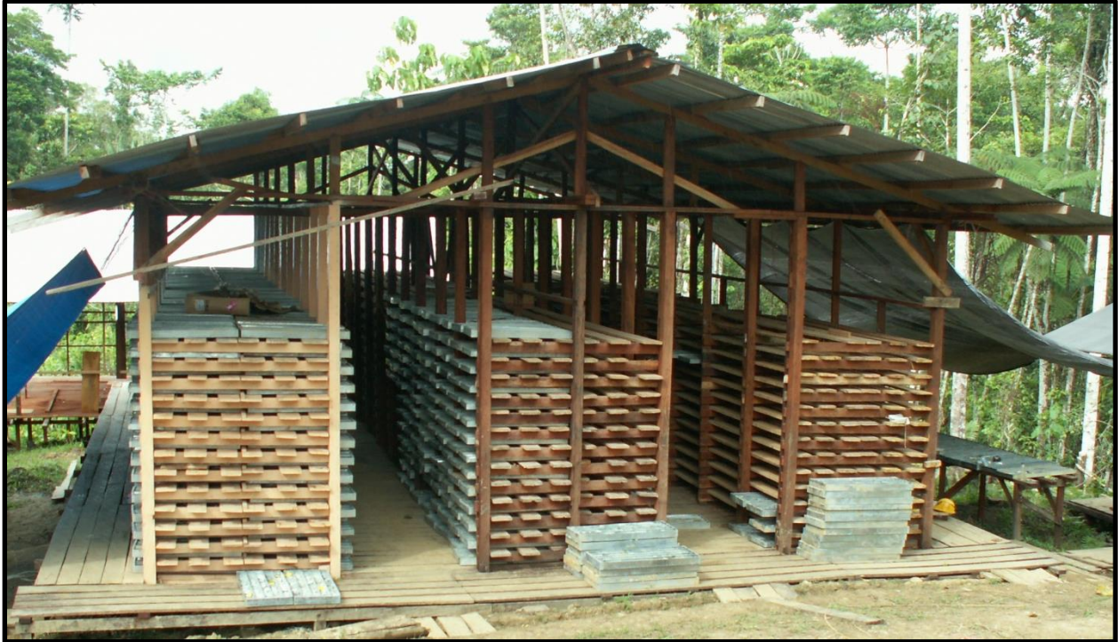
Photo 1. Neatly stacked coreboxes in Tekai coreshed at end of final drilling program on 27 March 2007.
