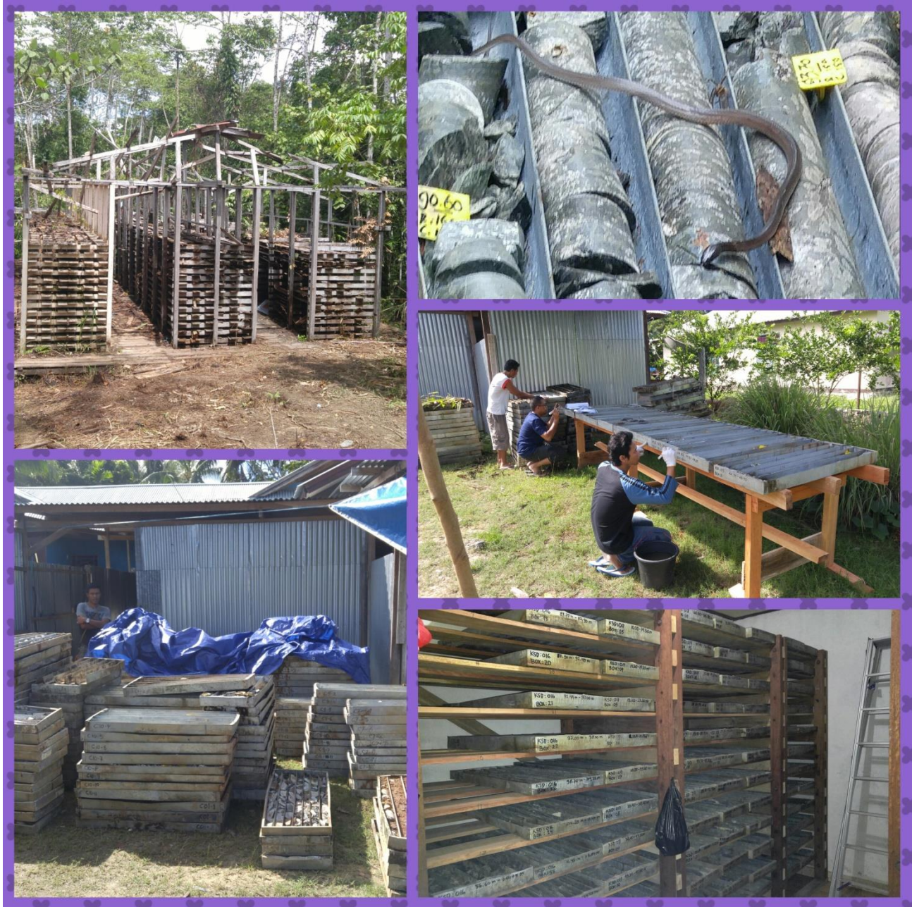
Photo 4 Clockwise from bottom left : coreboxes unloaded in Arso prior to sorting, completely empty coreshed at Tekai, last hurrah of a Tekai snake, re-labelling sorted coreboxes at Arso prior to re-photographing and re-stacking, coreboxes neatly stacked in order in shelves in new core storage facility at Arso.
