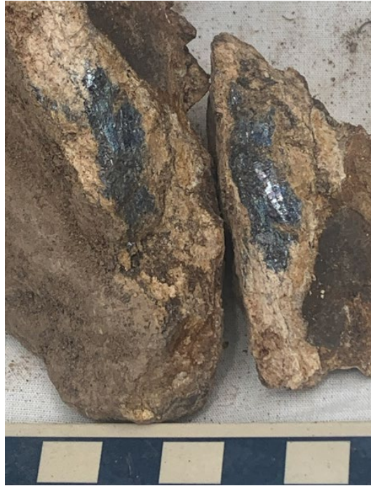
Sample MVS17: 52.3% Antimony and 0.08grams/tonne Gold. Vein of white-yellow-minor green antimony oxide (antimony trioxide Sb_2O_3 ), and silvery-grey antimony sulphide (stibnite, Sb_2S_3 ) up to 32mmx12mm, hosted in grey, silicified pelite. Note the acicular (elongate) stibnite crystals. Single rock collected from mine dump and fragmented for examination (scale bar: Centimetre divisions).
