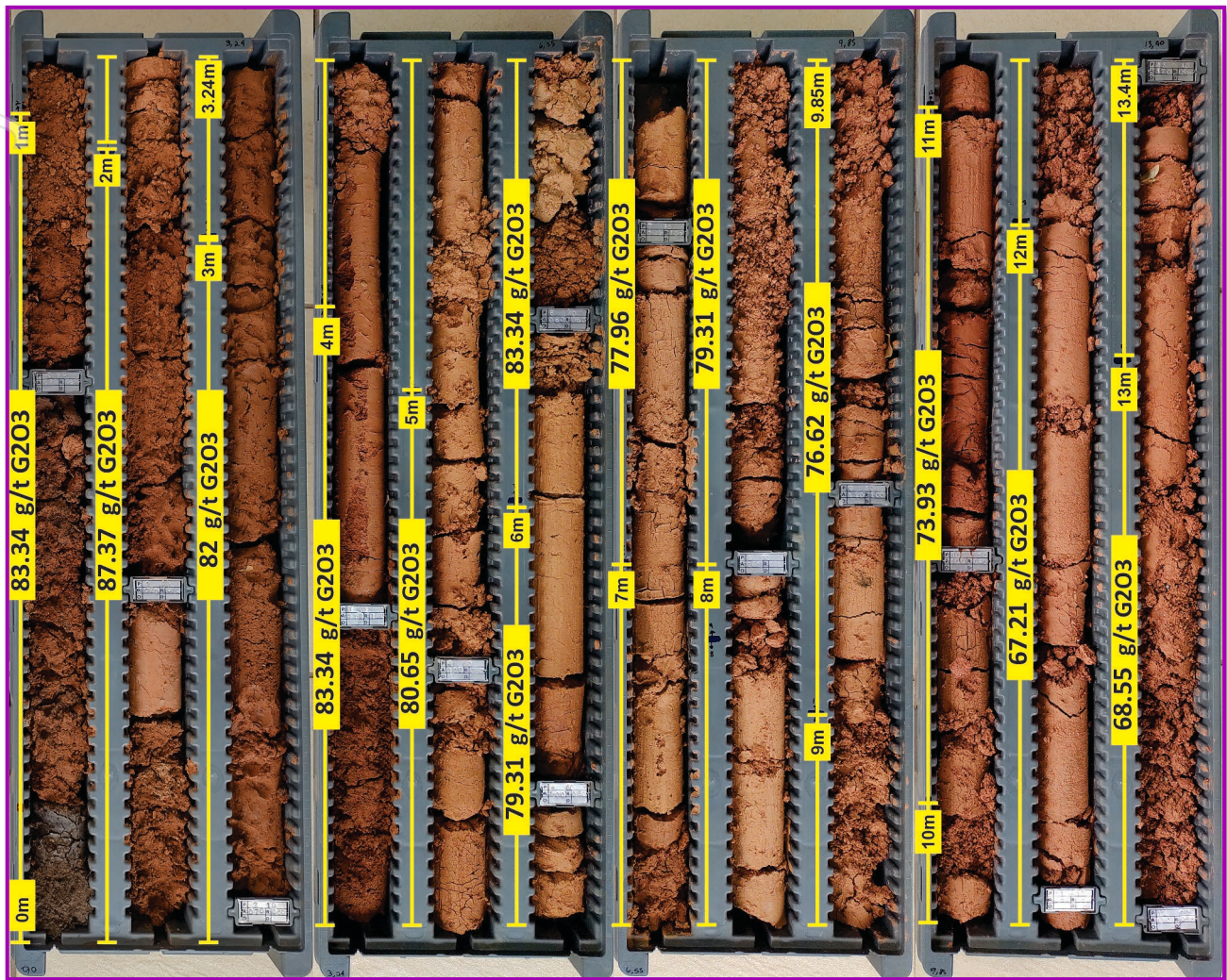
Figure 4 – CLD-DDH-005 diamond drill core showing high grade Ga 2 O 3 values in lateritic soil.
