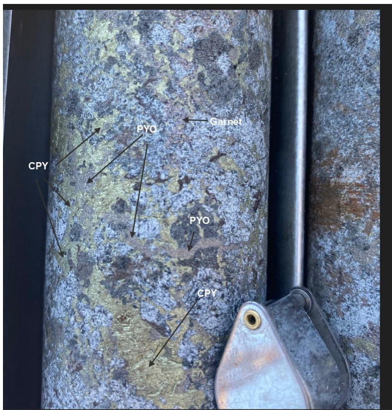
Figure 1: Copper sulphide mineralisation intersected within 608.00–609.00m interval in OFMSD083 with 2.69% copper and associated pyrrhotite and pyrite, which makes the mineralisation suitable for electrical geophysical methods. Detailed assay results are provided in Table 6.
