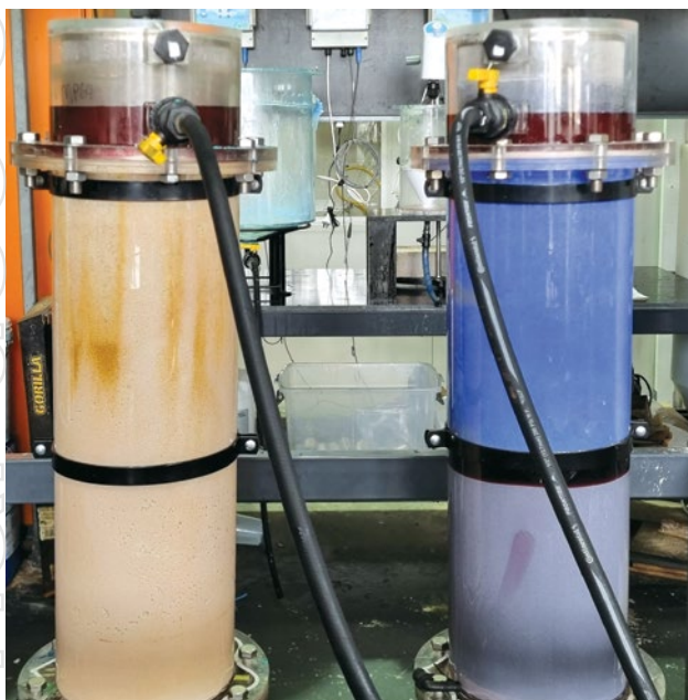
Figure 1 – Cobalt separation using a system of ion-exchange columns at the Broken Hill Technology Development Centre
