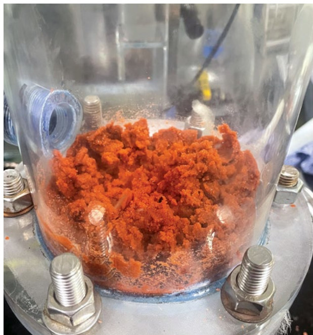
Figure 2 – Final product cobalt sulphate in the crystalliser
