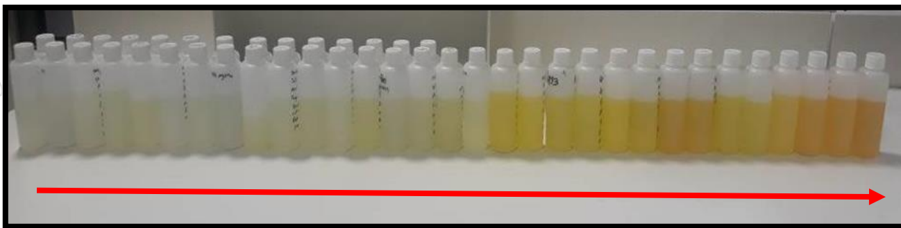
Figure 2: Visual changes during acid leaching process optimisation. The image illustrates the changes in sample colours (from left to right) resulting from the optimisation of various parameters during the acid leaching process, highlighting the effect of extracting different oxidation states of elements on the colour of the samples.
