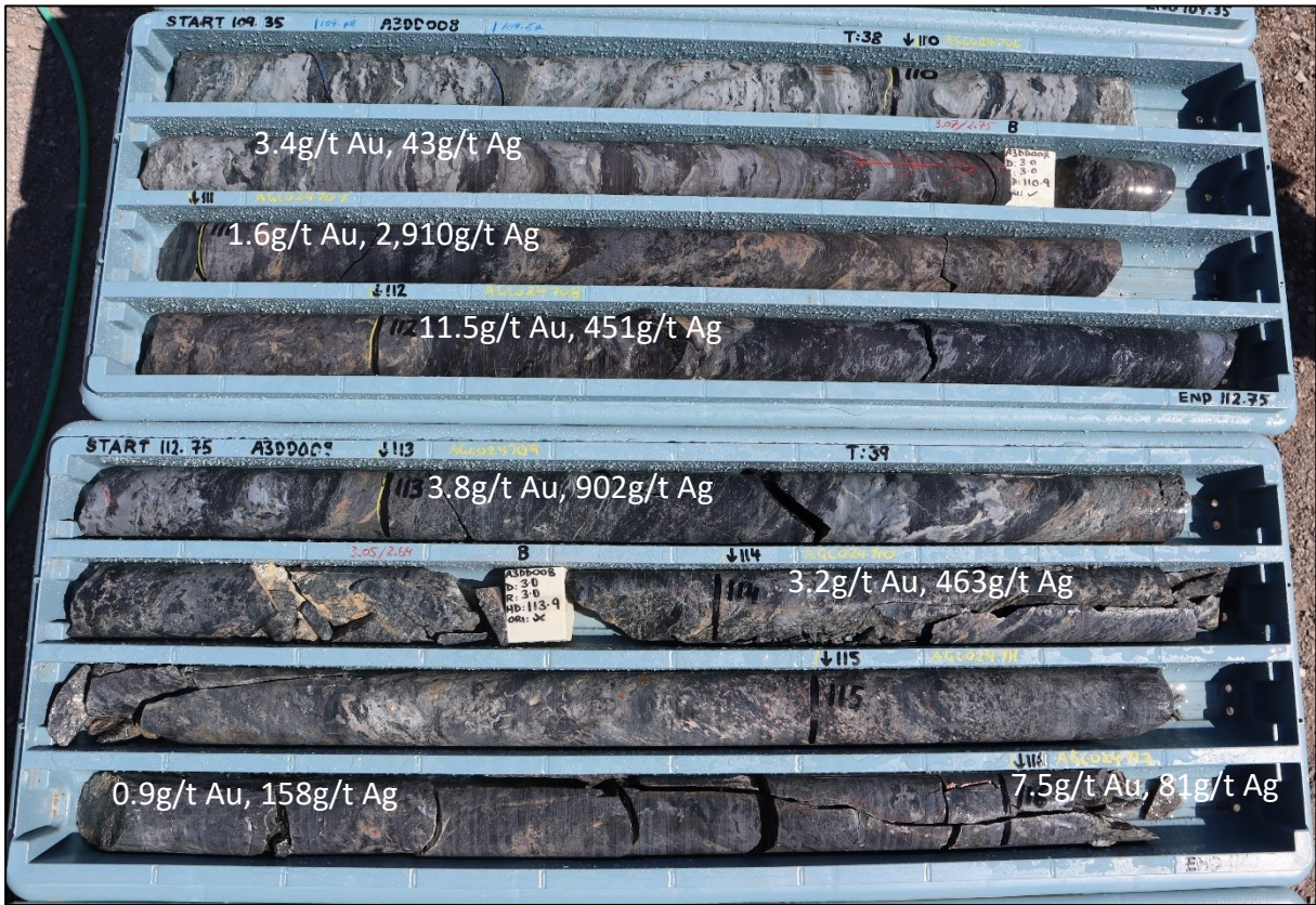
Figure 3: Core photographs of most of the 9m wide, high grade silver-gold zone in A3DD008 grading 3.7g/t Au, 566g/t Ag & 1.4% Pb+Zn from 110m.
