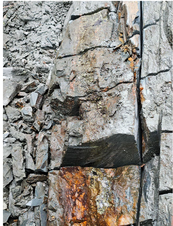
Figure 4: Chalcopyrite rich mineralisation, with associated quartz veining and orange-red potassic feldspar alteration
