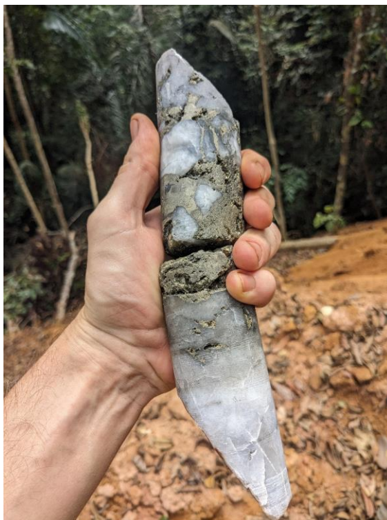
Figure 3: Mineralised veining in hole SLDD002 along trend from underground workings (sample P1586: 1.2g/t Au).
