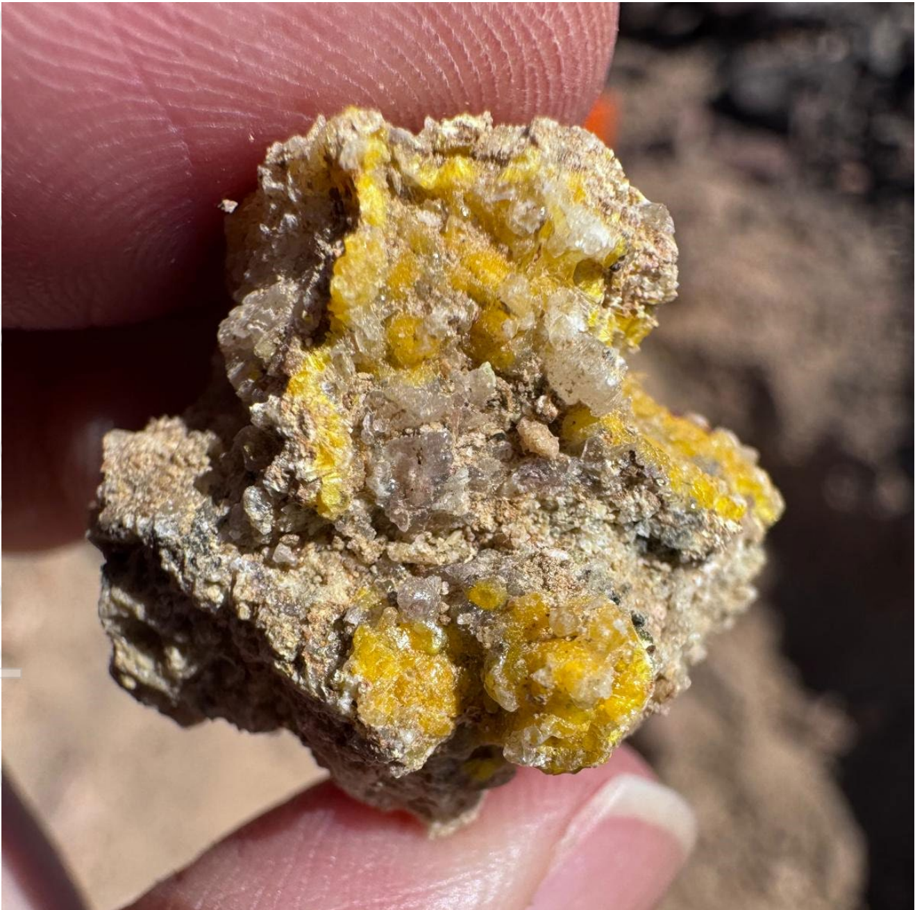
Figure 3. A field specimen of uranophane (a secondary uranium mineral) gathered from the site of sample CMRS4 at the Etango North-East Project
