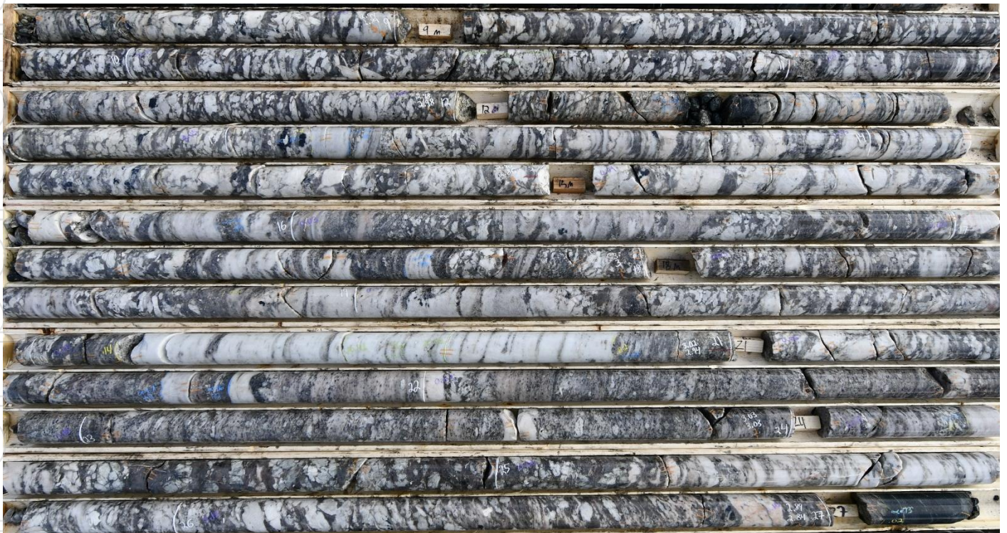
Figure 4: Pegmatite intercept 8-27m (18.7m intercept width) at 1.39% Li 2 O hole JD-24-001
