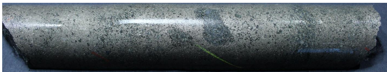
Figure 1: Massive pyrrhotite-pentlandite-chalcopyrite with rounded clasts of entrained norite, from a 0.64 m sample that returned 1.6% Ni, 0.2% Cu, 0.15% Co, 179.50 m, 24RAN010. NQ diameter drill core
