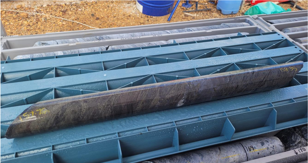
Figure 2: Photo of diamond drill core from GLPDD007 showing massive sulphide mineralisation at 157.75m grading into semi-massive sulphides with pyrite, sphalerite, galena and chalcopyrite (refer Appendix 1)
