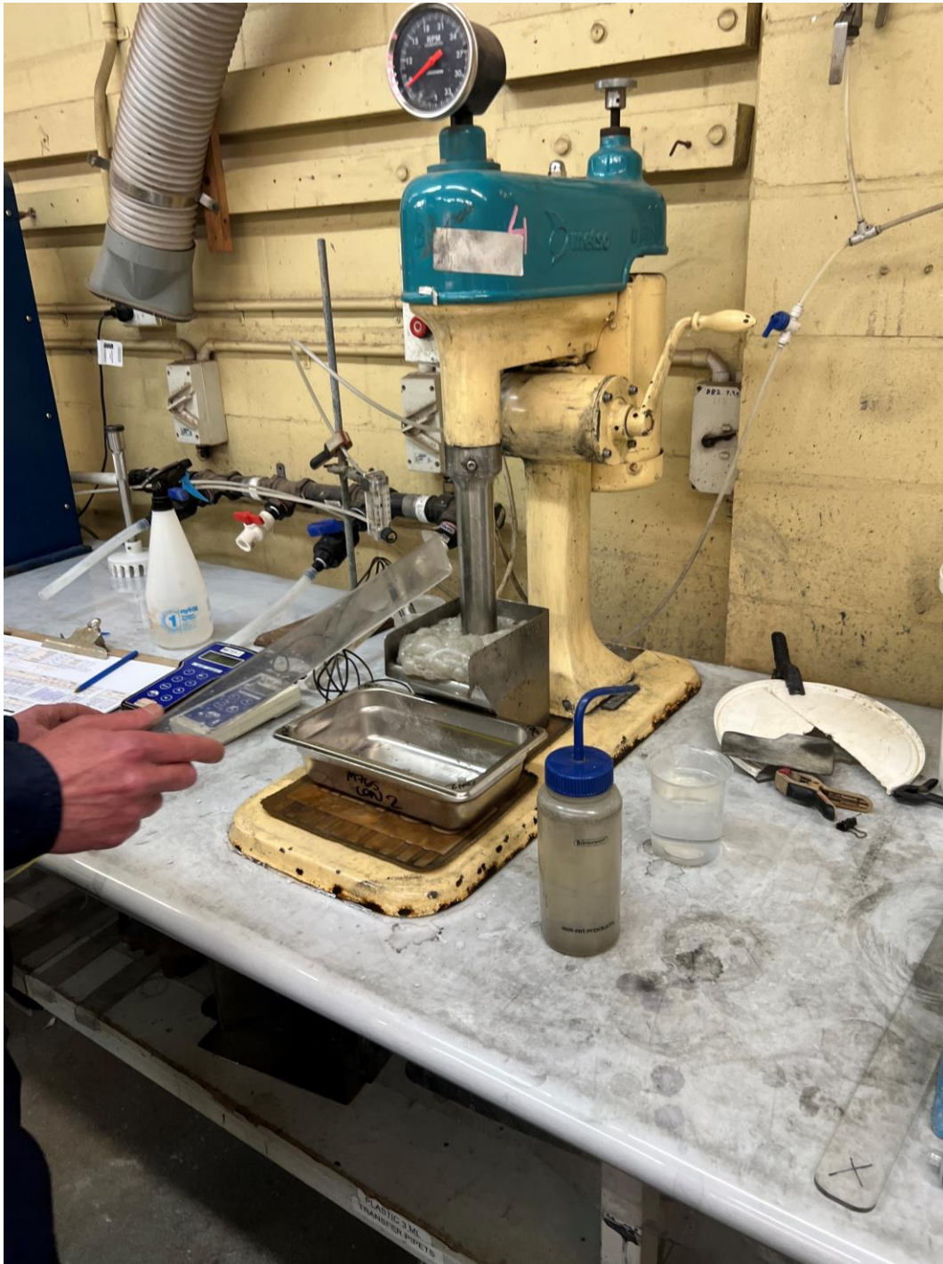
Figure 3 - Metso flotation unit used to recover lithium to a spodumene concentrate
