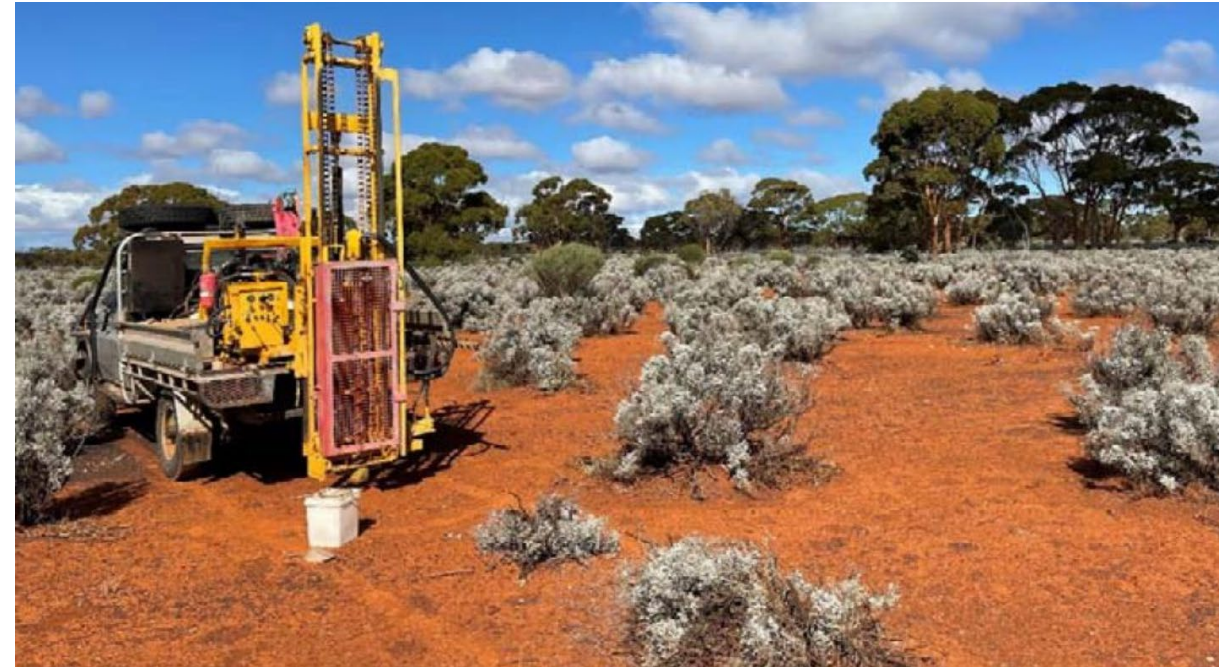
Auger rig used for calcrete sampling
