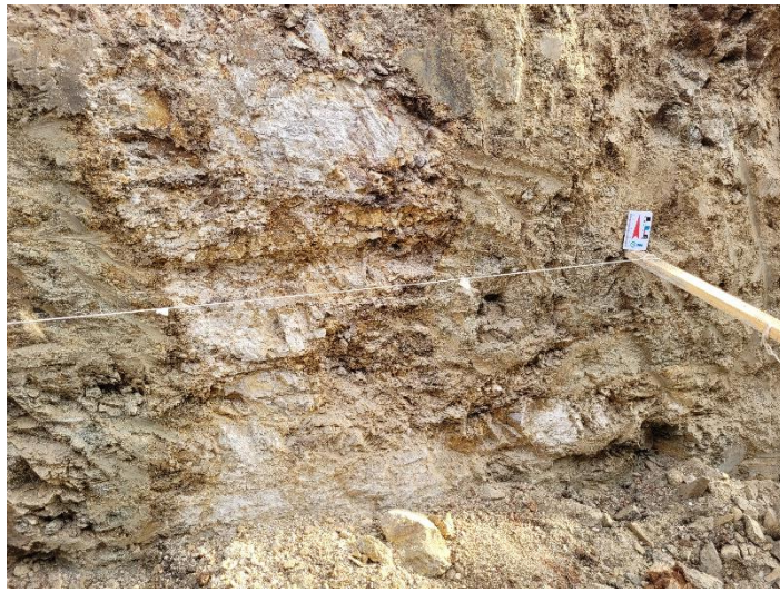
Figure 4 Exposed pegmatite dyke in trench TR-01, Feirinha Prospect. This is one dyke of a swarm of similar dykes mapped on the prospect.
