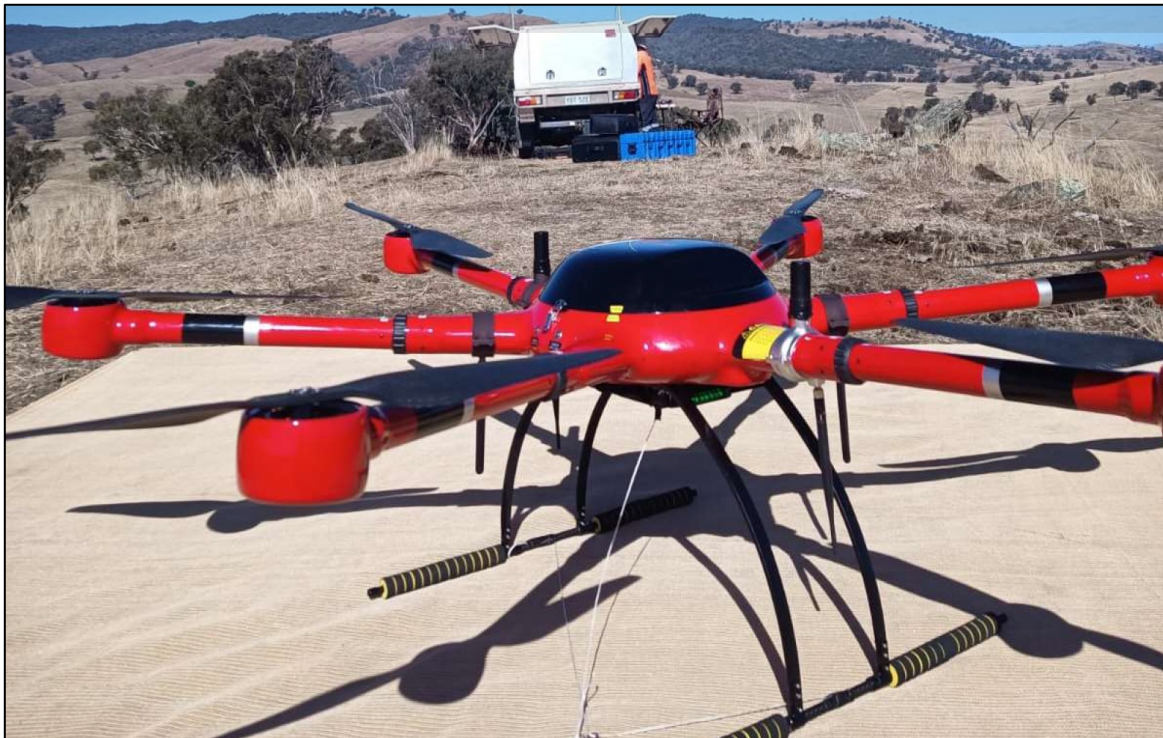
Figure 1: AirGeoX's six-rotor drone fitted with a magnetometer being readied for take-off.
