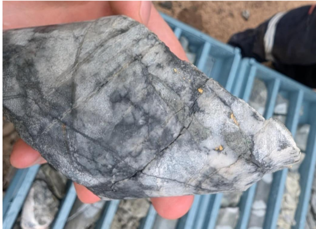
Picture 2: Quartz stibnite vein with coarse visible gold at 776.6 m. Interval assayed 0.16 m @ 3,330 g/t Au and 11.7% Sb from 776.6 m. Scale across image approximately 16 cm.
