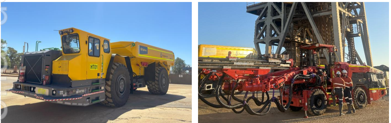
Figure 3. New Epiroc MT65 Truck (left) and Sandvik DD321 Drill (right).
