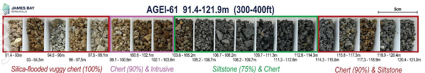
Figure 8: AGEI-61 drill chips (per sample interval) between 91.4 - 121.9m. Lithologies highlighted and approximate proportion of the dominant lithology displayed.
