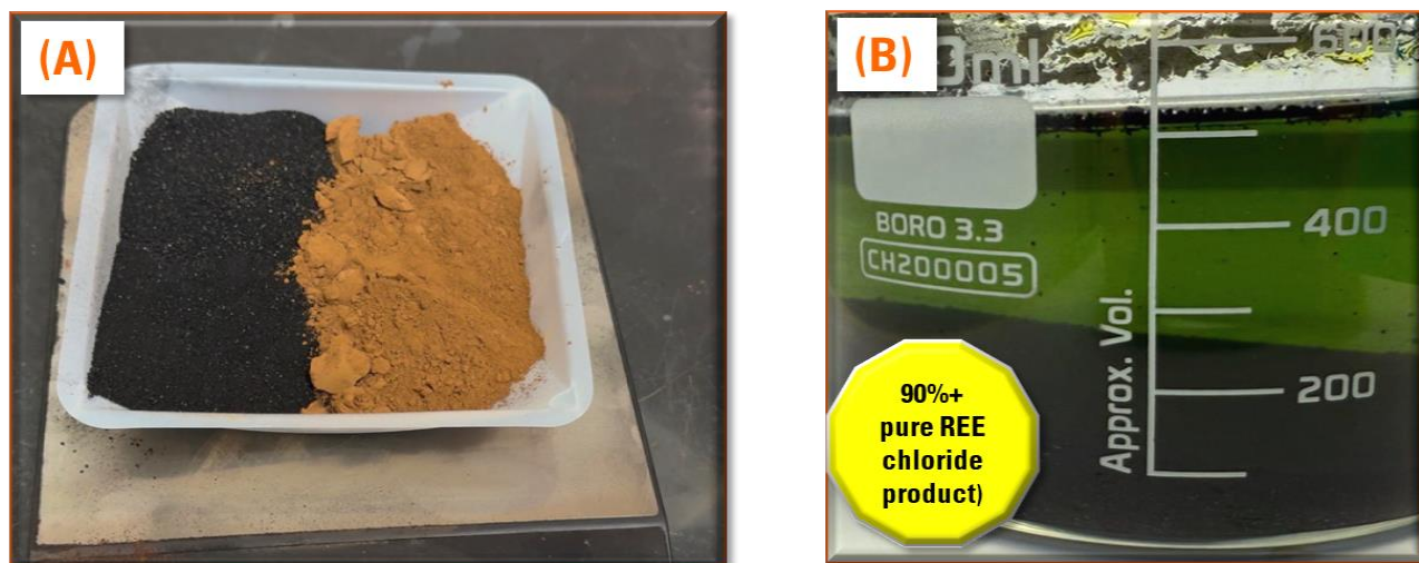
Figure 4: Photos of (A) Pre-Flash Sample of Feedstock (Flotation Concentrate) (RHS) with carbon (LHS), & (B) High purity REE-chloride product (>90% purity) produced from water-washing the post flashed solids
