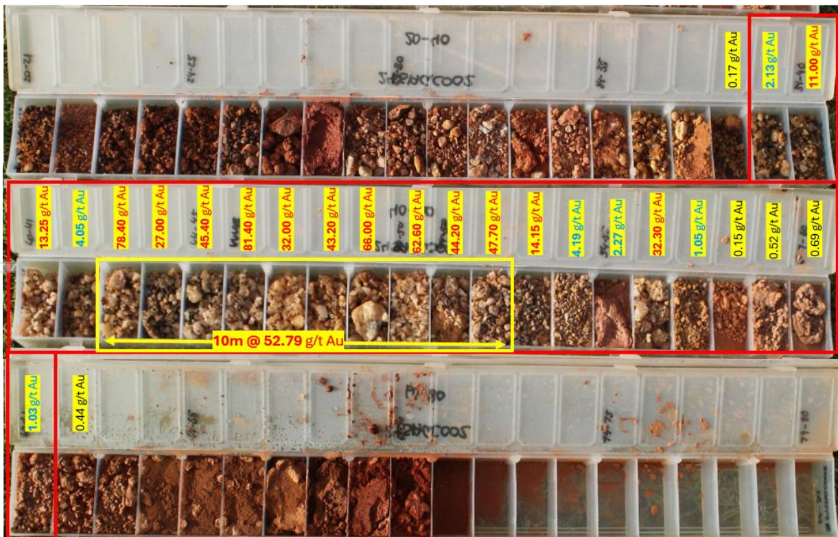
Figure 3: RC drill chips showing the quartz lode and bonanza gold zone, 23m @ 26.73g/t Au including 10m @ 52.79g/t Au , intersected in hole 24SAGC002.
