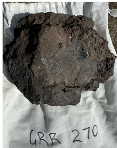
Figure 4: High-grade massive black manganese oxide mineralisation, 53.50% Mn, Sample GRR270
