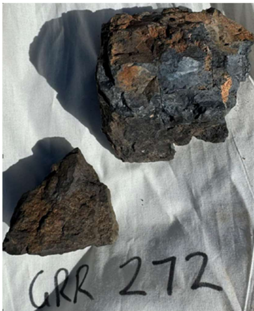
Figure 3: High-grade massive black manganese oxide mineralisation, 54.50% Mn, Sample GRR272
