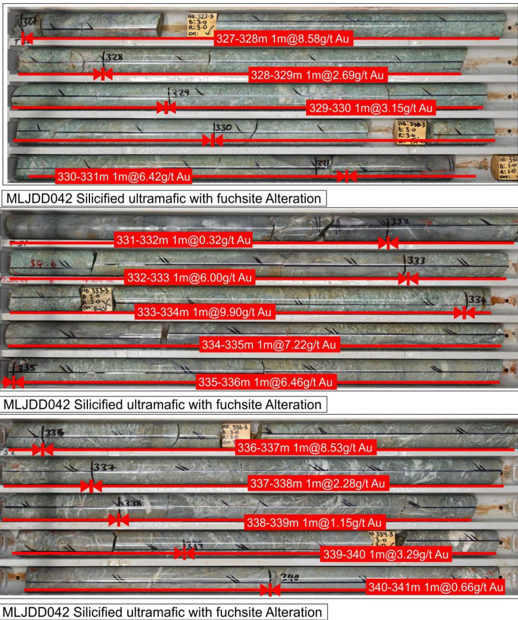
Figure 12. Drillhole MLJDD042 from 327m to 341m showing silicified ultramafic with fuchsite alteration
