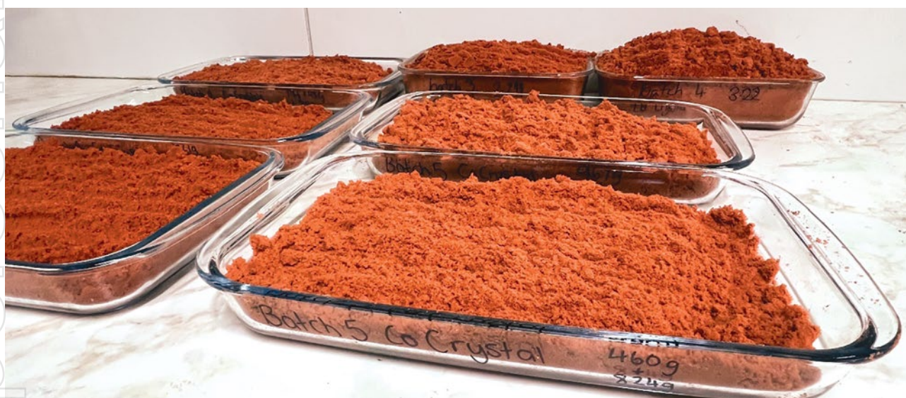
Figure 2 – Cobalt sulphate produced at the Broken Hill Technology Development Centre Plant
