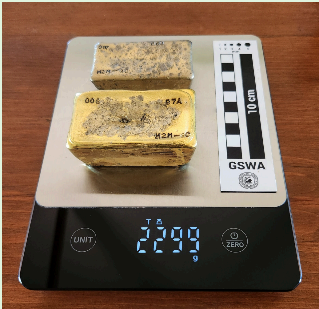
Picture 1. Picture of Gold doré bars produced from Batch- B6 B and B7A.
