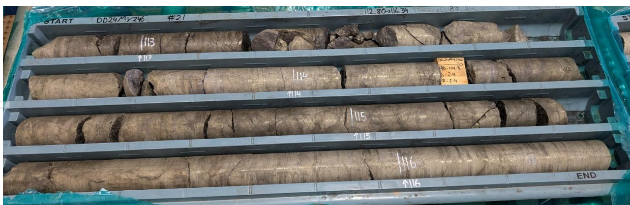
Figure 1: DD24MY246: massive pyrite-chalcopyrite-galena mineralisation approximately 113m downhole
