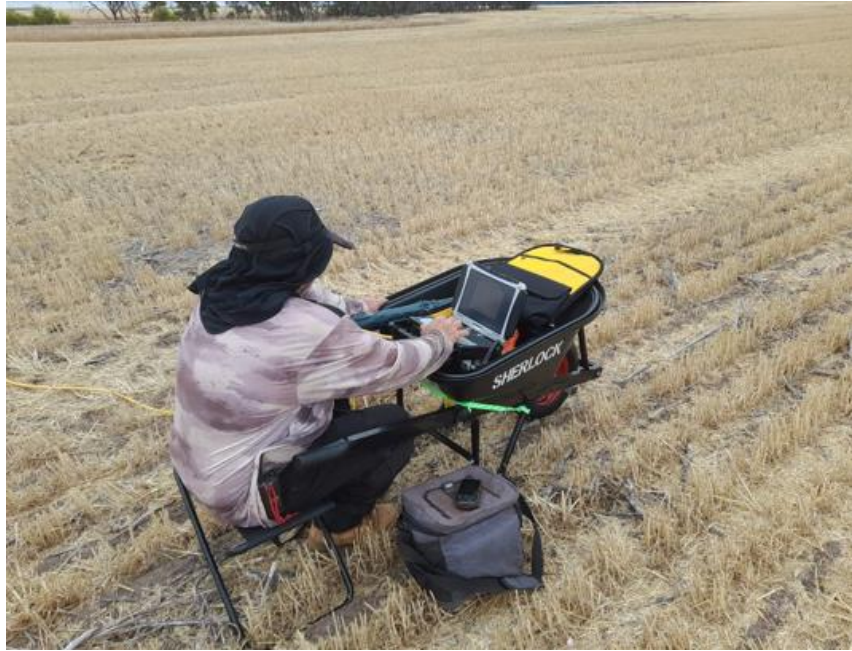
Picture 1. Ground EM survey over Targets 1 & 2 (refer to diagram 3), at the Lort River Vtem bedrock sulphide conductors. Operator above taking readings from the middle of each of the laid-out square wire loop station, refer to picture 2 for additional survey explanation.
