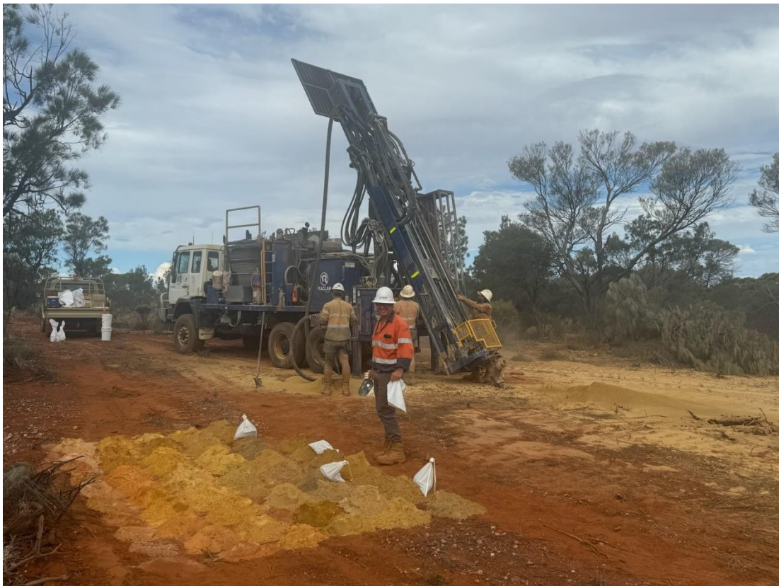
Figure 1: Aircore drilling rig Mulgabbie North
