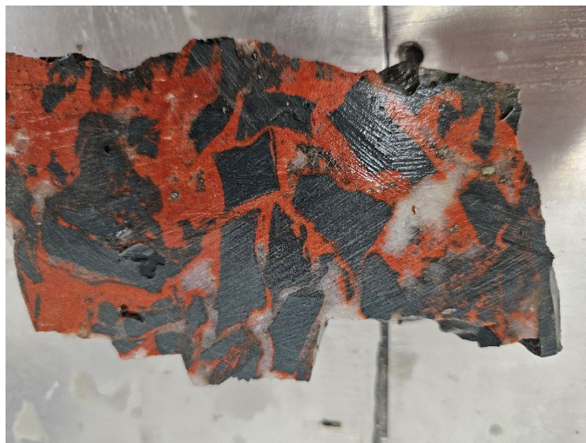
Figure 5: Brecciated host shale with infill of quartz and intense potassic feldspar alteration (orange-red) and sulphide aggregations. Estimated sulphides 5%**
