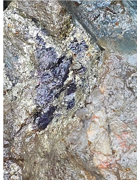
Figure 7: Chalcopryite-pyrite-pyrrhotite-covellite(?) massive sulphide vein at the Chevrier Prospect. Photo width 50cm. Estimated 70% sulphides within vein**.
