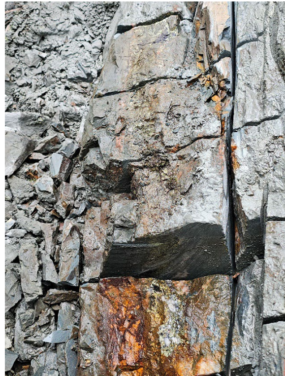
Figure 4: Chalcopyrite rich zone within Chevrier adit, with associated quartz veining and orange-red potassic feldspar alteration. Estimated 40% sulphides in mineralised zone**
