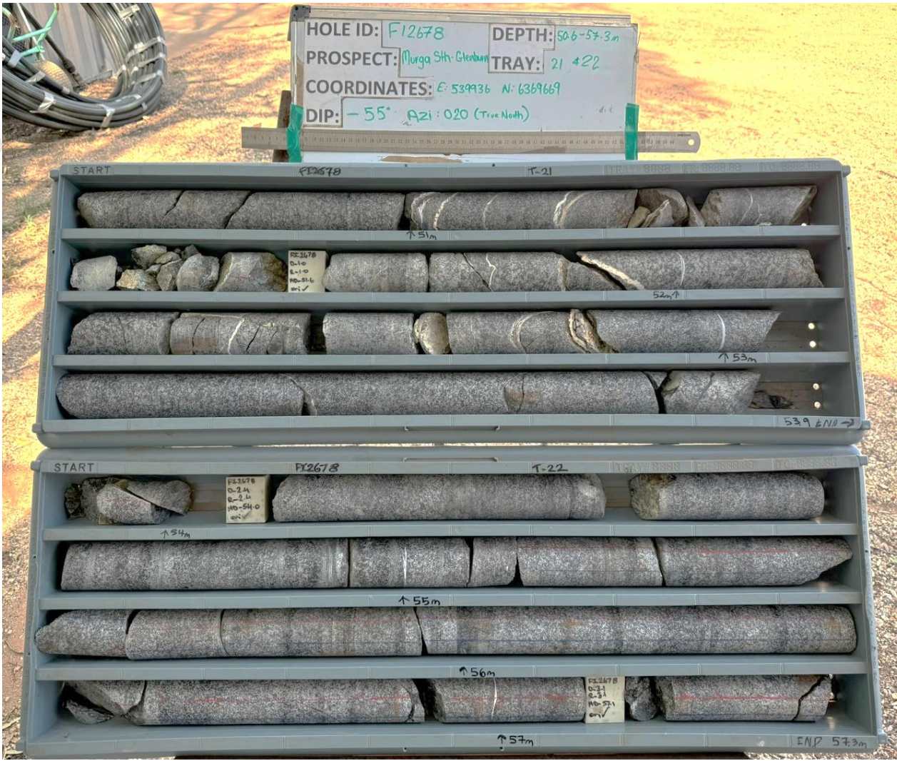
Figure 4: Photo of FI2678 HQ core – 50.6 to 57.3 metres (coarse grained pyroxenite)
