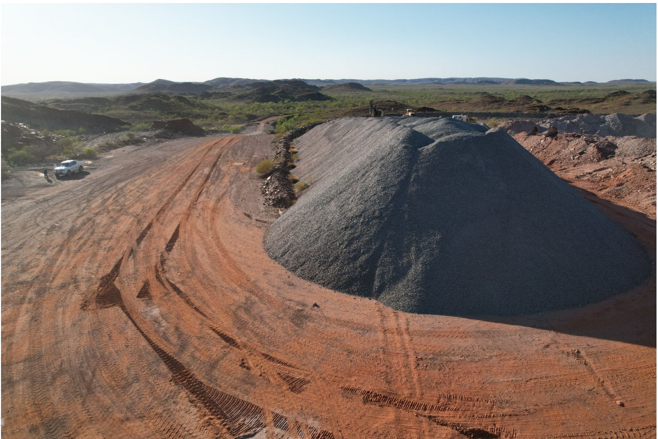
Figure 6: Commercial scale waste rock to road base trial product
