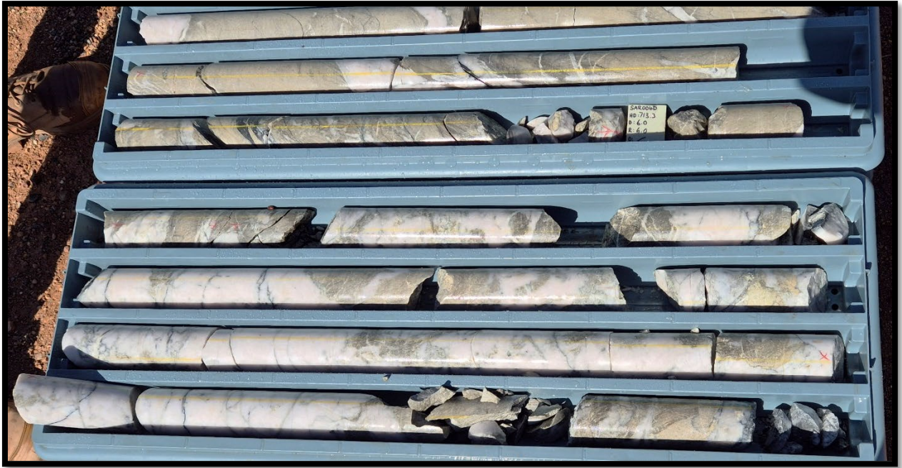
SAR004D (711m – 717m) – Quartz veined sericite-carbonate altered monzodiorite with arsenopyrite-pyrite selvage mineralisation. Interval graded 6m at 1.37g/t Au from 711m.
