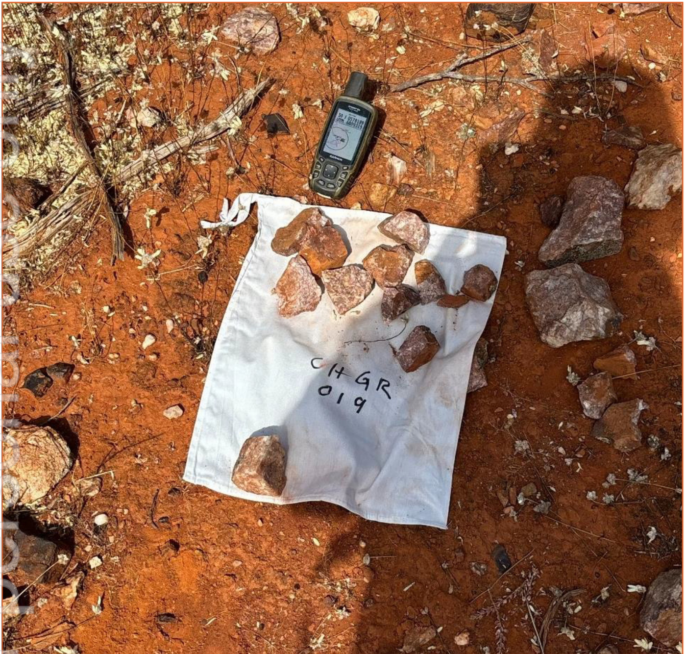
Figure 5: Sample number CHGR019 rock chips recording 1.0g/t Au
