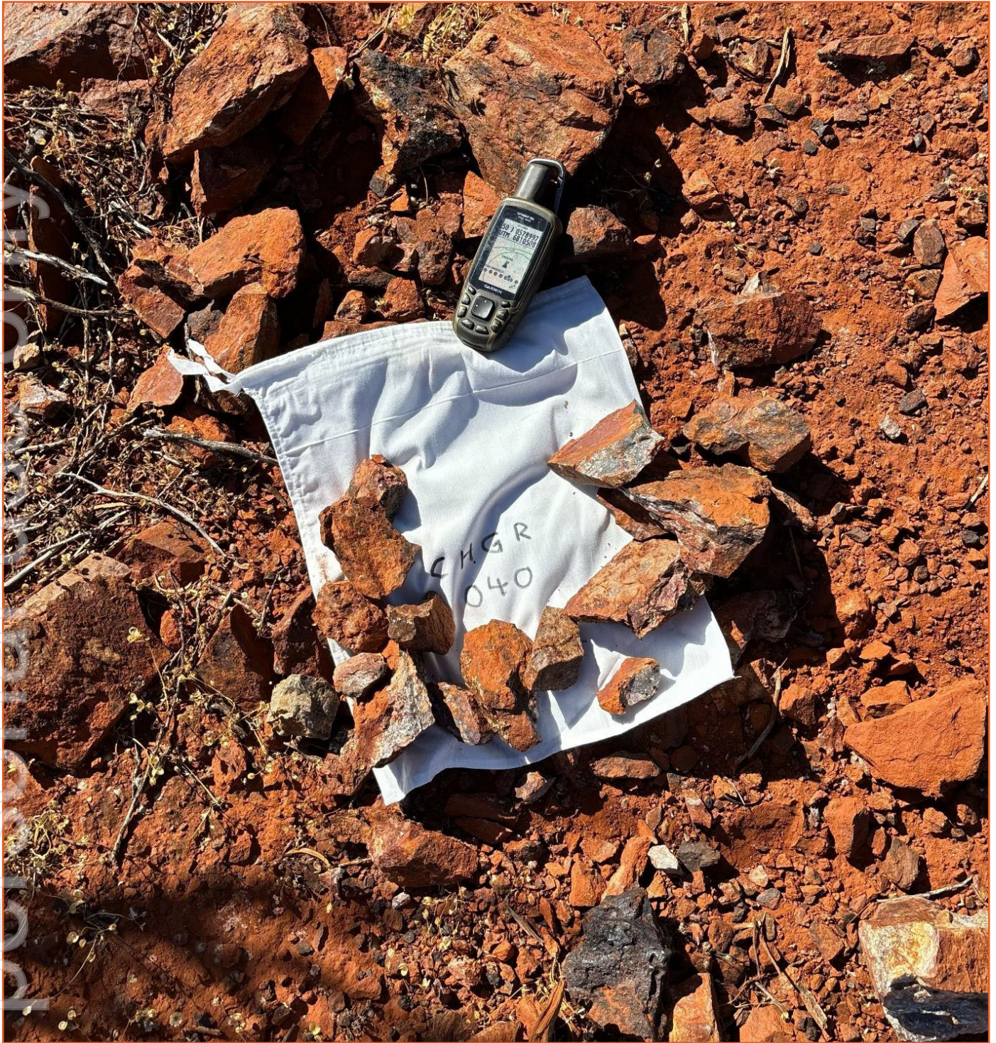
Figure 6: Sample number CHGR040 rock chips recording 0.91g/t Au
