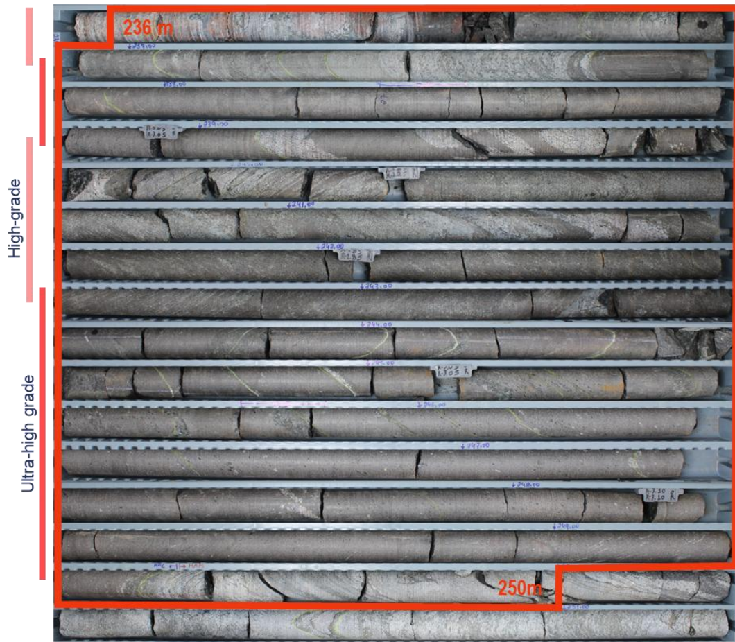
Figure 6: MADD0106: 14m at 21.3% TREO from 236m, including 6.4m at 28.9% TREO from 243m
