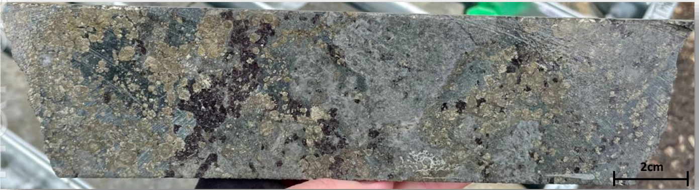
Figure 5. Core photo of polymetallic mineralisation from 574.4 metres in ZRSD24166. Laboratory assays returned 2.2g/t Au, 1.6% Cu, 0.4% Pb, 0.4% Zn. Common mineralogy includes chalcopyrite (bright yellow), galena (grey), pyrite (light yellow), pyrrhotite (brassy/bronze) and sphalerite (dark brown/black).
