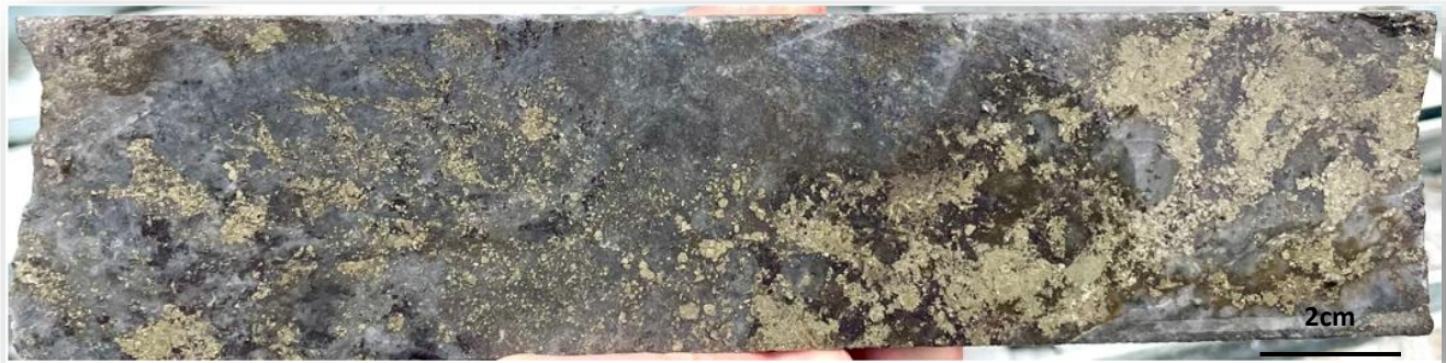
Figure 1: Core photo of polymetallic gold-copper mineralisation from 503.7m to 503.9m in ZRSD24166. Laboratory assays from this sample returned 1.0g/t Au, 0.5% Cu, 0.4% Pb, 1.1% Zn. Common mineralogy includes pyrite (light yellow), chalcopyrite (bright yellow), galena (grey), pyrrhotite (brassy/bronze) and sphalerite (dark brown/black).
