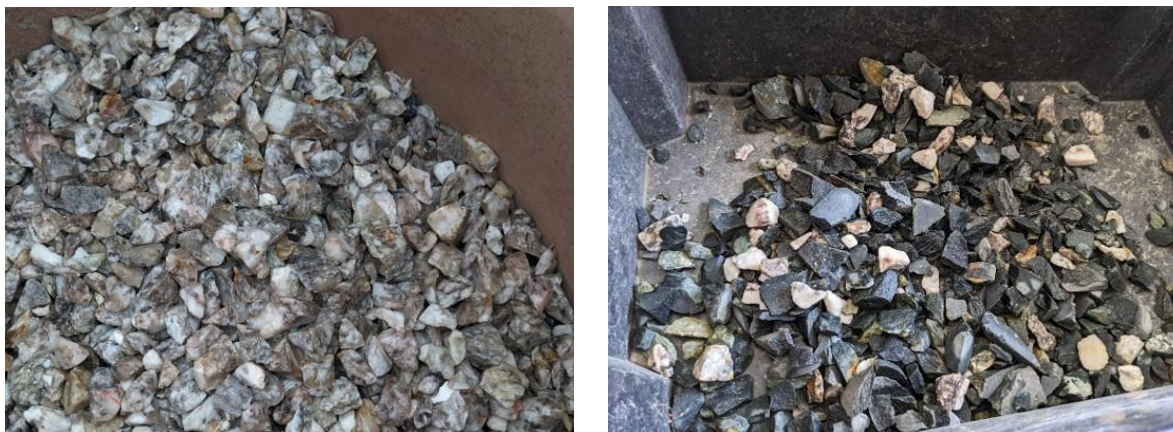
Figure 3 – Typical ore sorter products, pegmatite on the left to ore feed and basalt, feldspars and quartz on the right to waste. The photographs are of samples generated in-train and are therefore incomplete. Assays of the final products for each composite sample run are shown in Table 2.
