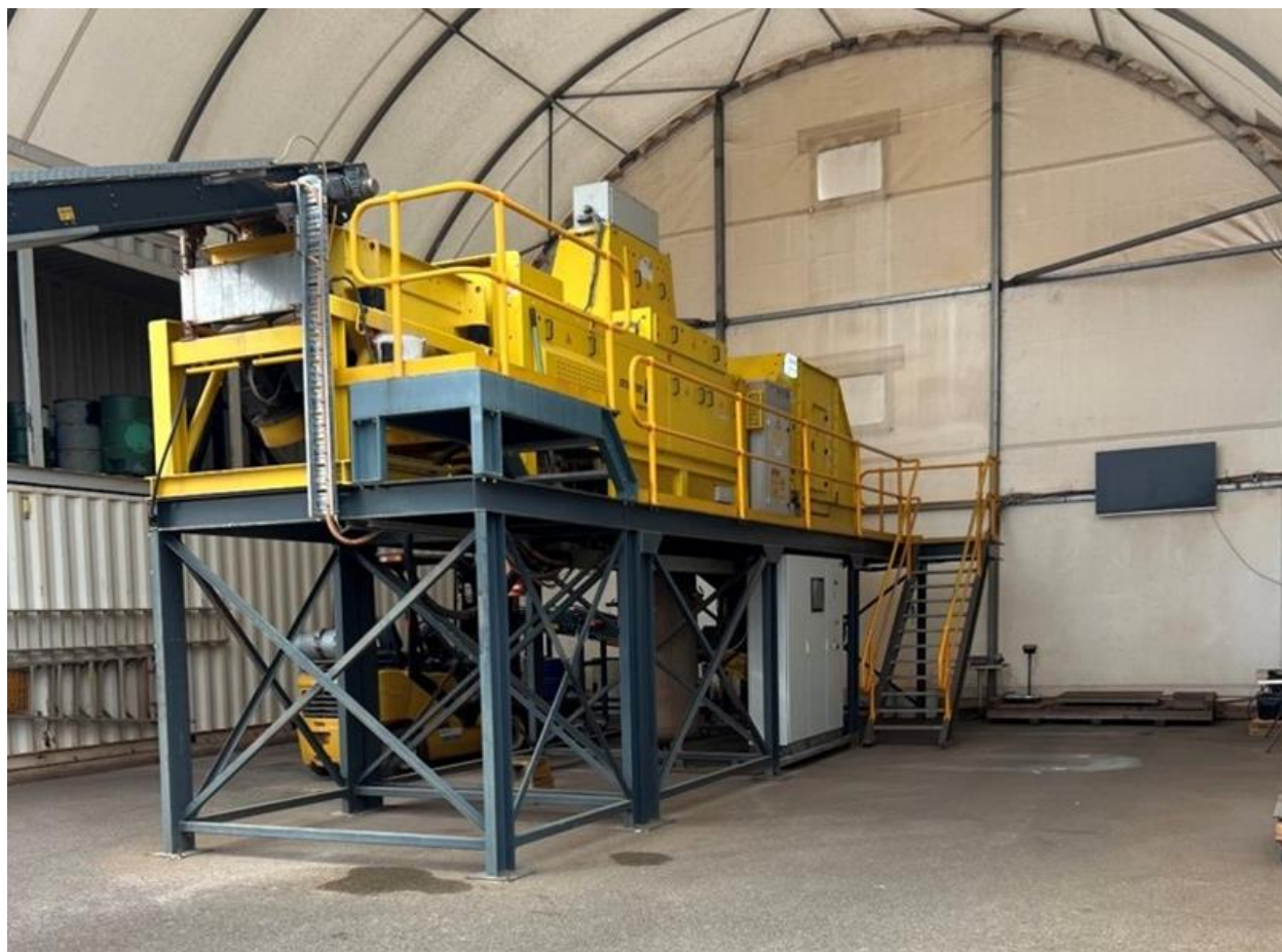
Figure 2 – Steinert Ore Sorter used in the testwork
