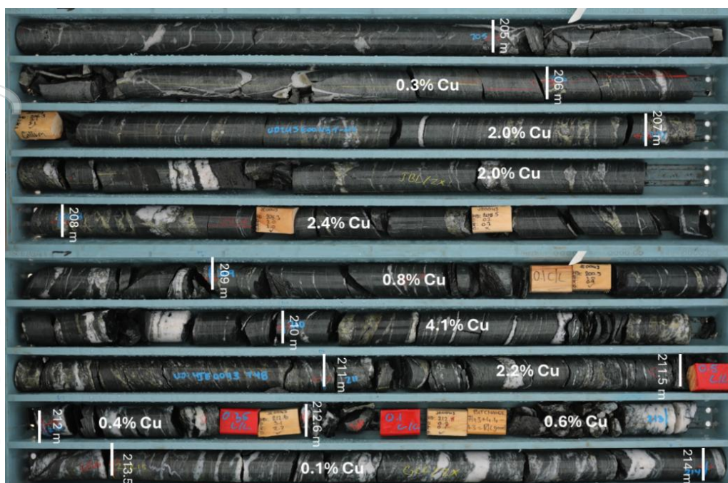
Figure 7: A section of Jubilee North drillhole UD24JE0043 highlighting 5.5m at 2.3% copper from 206m.
