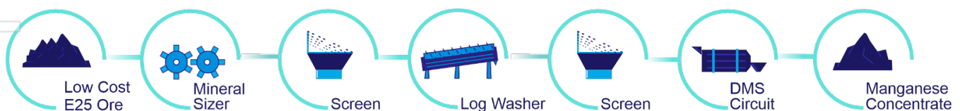
Figure 5: Simplified Process Flowsheet
