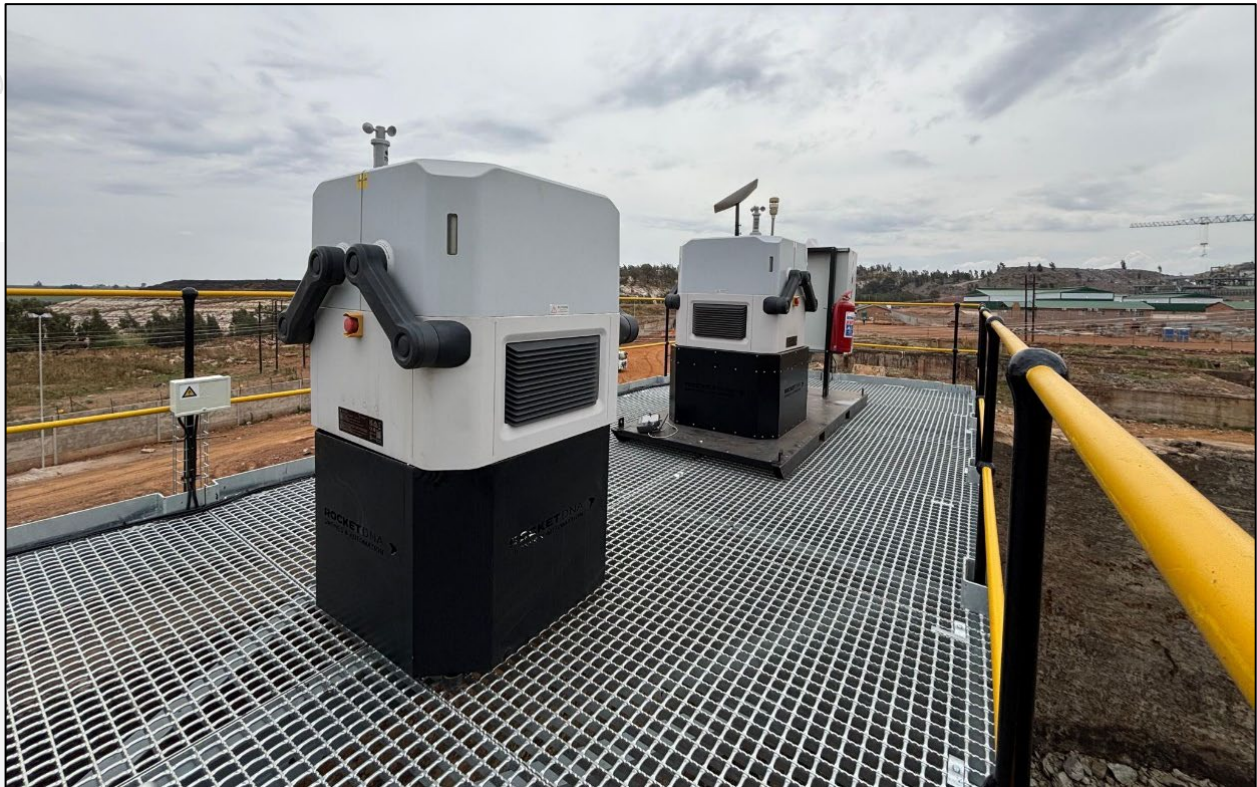
Figure 1: RocketDNA's xBot® - a fully configured and integrated remote drone docking solution, operated remotely from our Remote Operating Centre using AI-enabled software for security, inspections, emergency response, mapping and more. No pilot onsite; installed in Africa.
