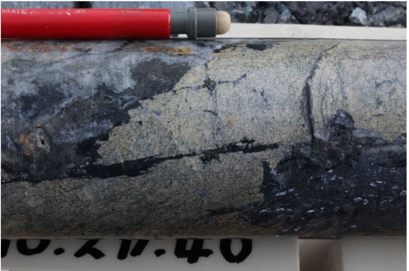
Photo 1: BHD006 (previously reported) 258.5m vein showing massive galena, Fe poor sphalerite, Mn oxide after rhodochrosite and Ag rich sulfosalt minerals. 6
