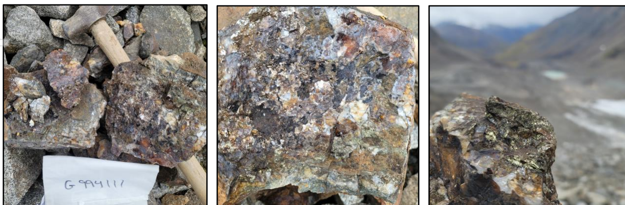
Figure 5. Stoney Vein sample G994111 – 6.1 g/t Au, 124 ppm Ag, 2.4% Cu, and 340 ppm Sb
