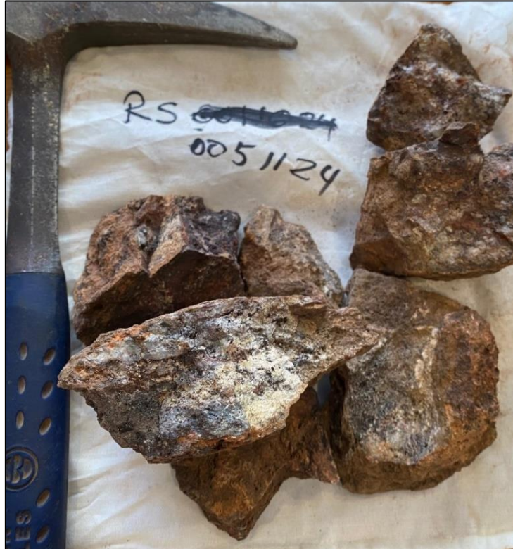
Figure 5. Sample R0051124 from Appaloosa showing iron oxide stained quartz veins in gabbro
