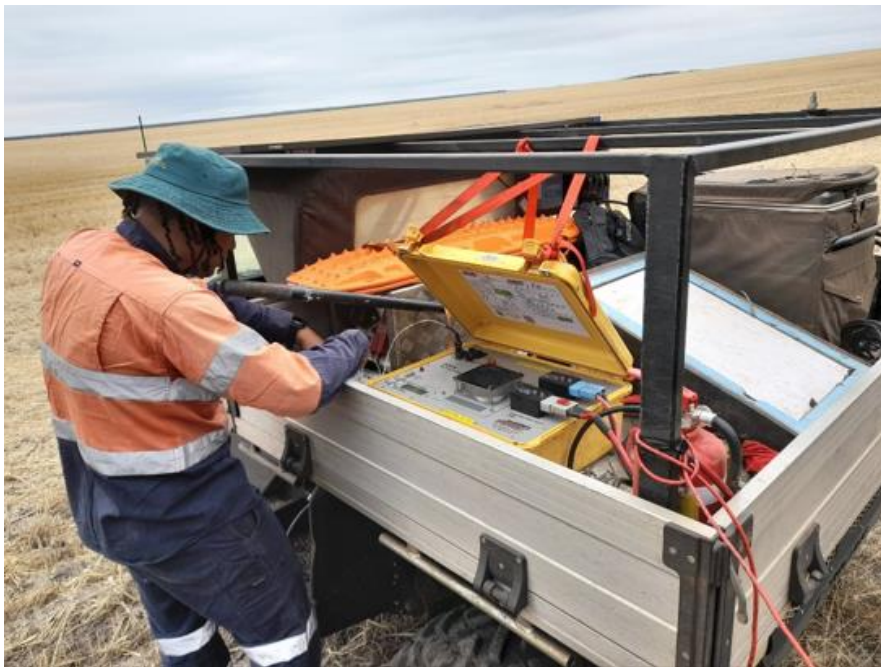
Picture 3. Ground EM survey at Lort river Project. Above picture is of one of the two EM survey operators, (other team member of the three positions cables) who is located at one corner of the actual on ground wire loop (8 or 10mm copper cable), the cables are laid out on the ground in a large 200m square loop. The above vehicle has a large battery and via the charge station (yellow box) the operator charges the loop with a measured electric charge, this charge creates a magnetic field throughout the wire loop, and it is this magnetic field that induces a response from present sulphides in the ground (if any are present). It's this magnetic (induced polarization) that the reading station located in the middle of the wire loop reads/measures. Each loop overlaps the next loop in the middle, across the whole target area.
