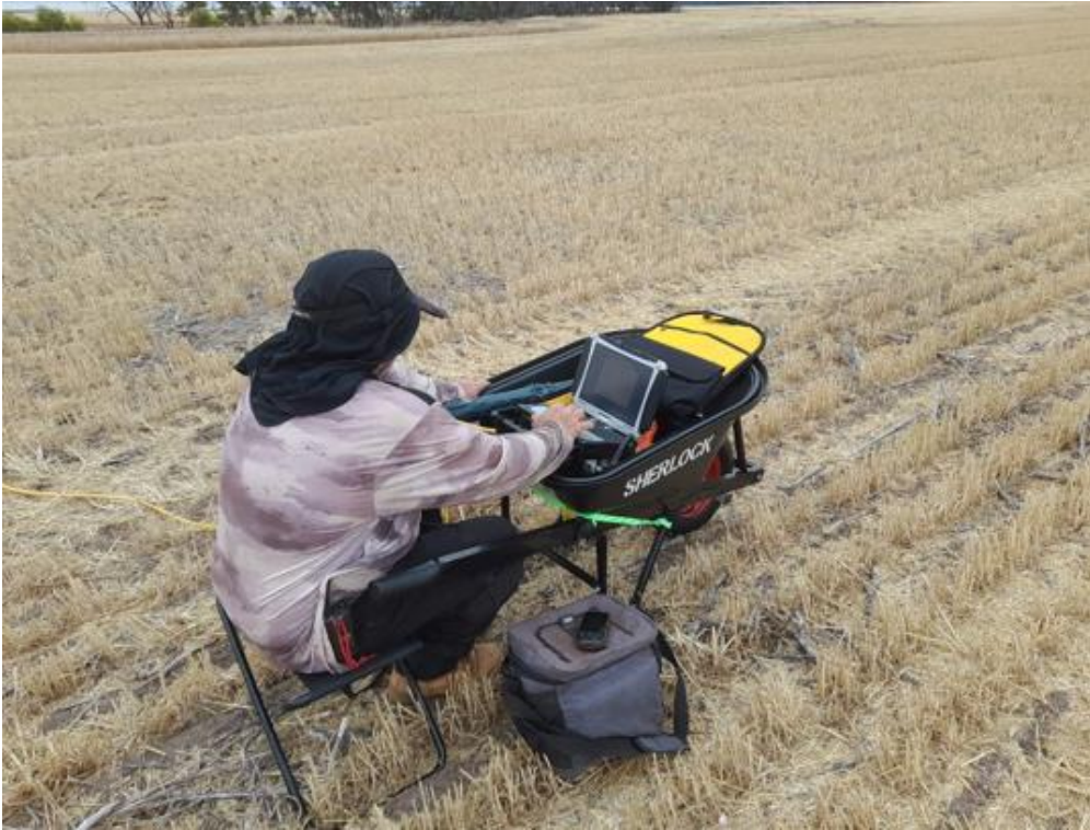
Picture 2. Ground EM survey over Targets 1 & 2, at the Lort River Vtem bedrock sulphide conductors. Operator taking readings from the middle of each of the laid-out loop (wire) station, refer to picture 3 for additional survey explanation.
