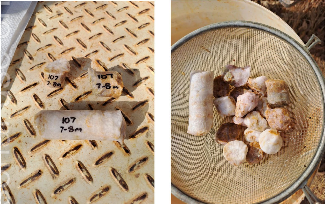
Figure 3: Quartz veining consistent with known mineralisation styles from the Northern and Central Targets on the Alice River Project, recovered from Aircore drillhole ARAC-1071
