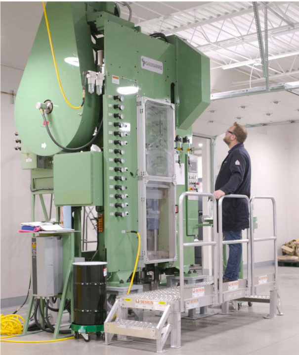
Figure 3 (clockwise from left): 100 ton uniaxial hydraulic press operations; Pre-HSPT fastener (LHS) and post- HSPT and threaded fastener (RHS); Pre-HSPT bars / pucks.
